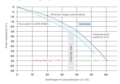
Special Antifrogen N antifreeze testers and refractometers are available for determining the frost resistance.
